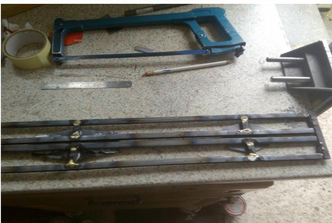
The problem of producing a pivot and bogie frame can be easily solved using the same techniques. The next shot shows the saddle drilled to take a “lazy susan” ball bearing plate. On to this are then riveted two U sections of Aluminium, L shaped brackets are then riveted to them. This gives a double beam cross piece -then you can rivet the bogie plate to it. Reversing the system gives a movable bogie plate for a fully compensated bogie.
