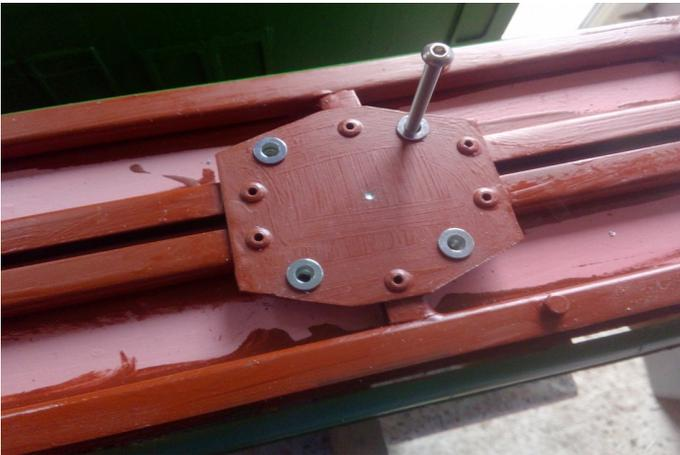
To make a simple removable fixing for the lazy susan you can use a “rivnut” that will insert a threaded length into a sheet section. The ones shown here are M4. So, as you can see the modern rivet gun is not to be disparaged as a butchers tool and can rapidly produce parts and assemblies for the railway.
